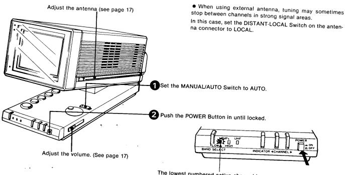
The lowest numbered active channel in your area will automatically be received and the red VHF Band Indicator will light.
